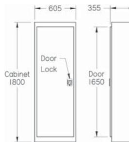
Fabricated from metal & powdercoated, to withstand the external elements, the cabinet is mounted at the ground level for easy access for emergency & maintenance purposes.
