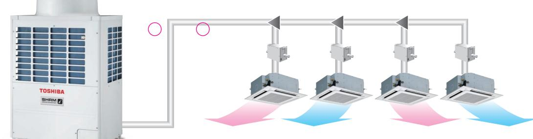
Recovered energy generated by the operation of indoor units is efficiently reused to heat and cool other zones.
