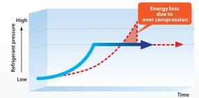
Superior partial load efficency with rotary compressor
