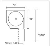
"B" = PELMET BOX HEIGHT AND DEPTH OAH = OVERALL HEIGHT (height from top of box to floor)
