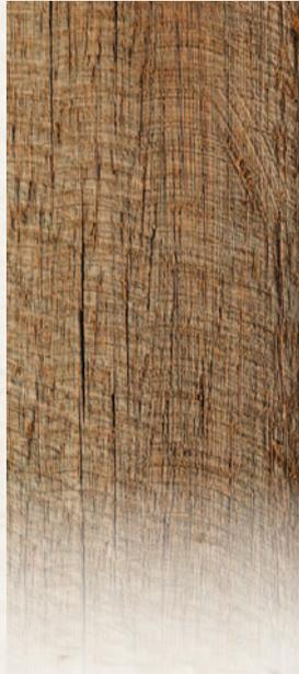
This finish is produced when large timber is sawn resulting in square or rectangular cross sections.
