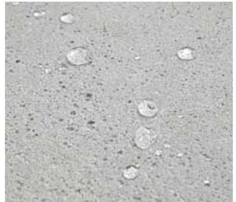
This concrete surface was sealed with a penetrating sealer, making it resistant to liquids.
