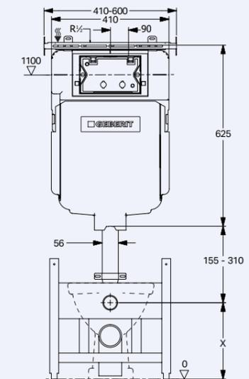
In-wall cistern installation diagram shown. For in-ceiling and in-duct installation diagrams, please visit the Download Centre at [geberit.com.au](http://geberit.com.au) and search 'remote button installation' or call 1800 GEBERIT.
