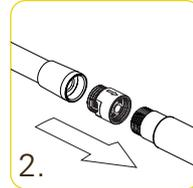
2. Install the Oxijet™ and ensure seal is attached between fittings
