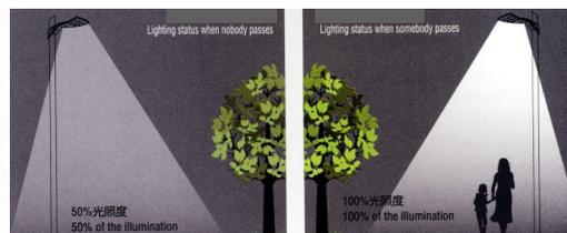
Optical sensor control. Reduces the power to 50% when nobody passes by, and increases to 100% when someone passes within the 10 metre sensing range
